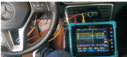
Power CAN bus communication
